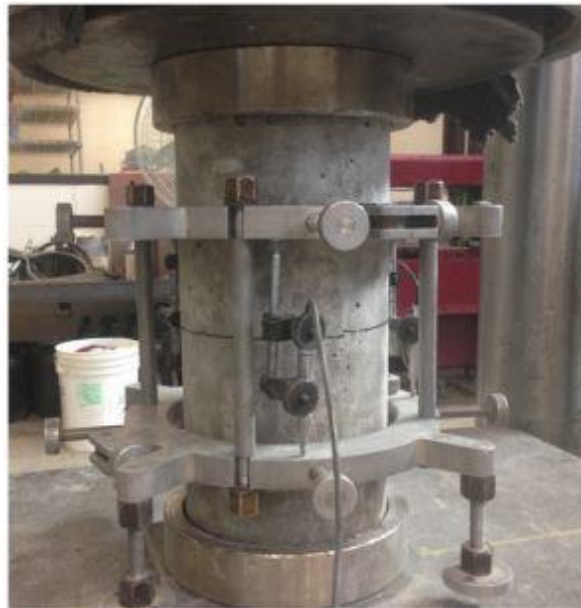
Figure 2.8: E-value Testing Arrangement for Cylinders
