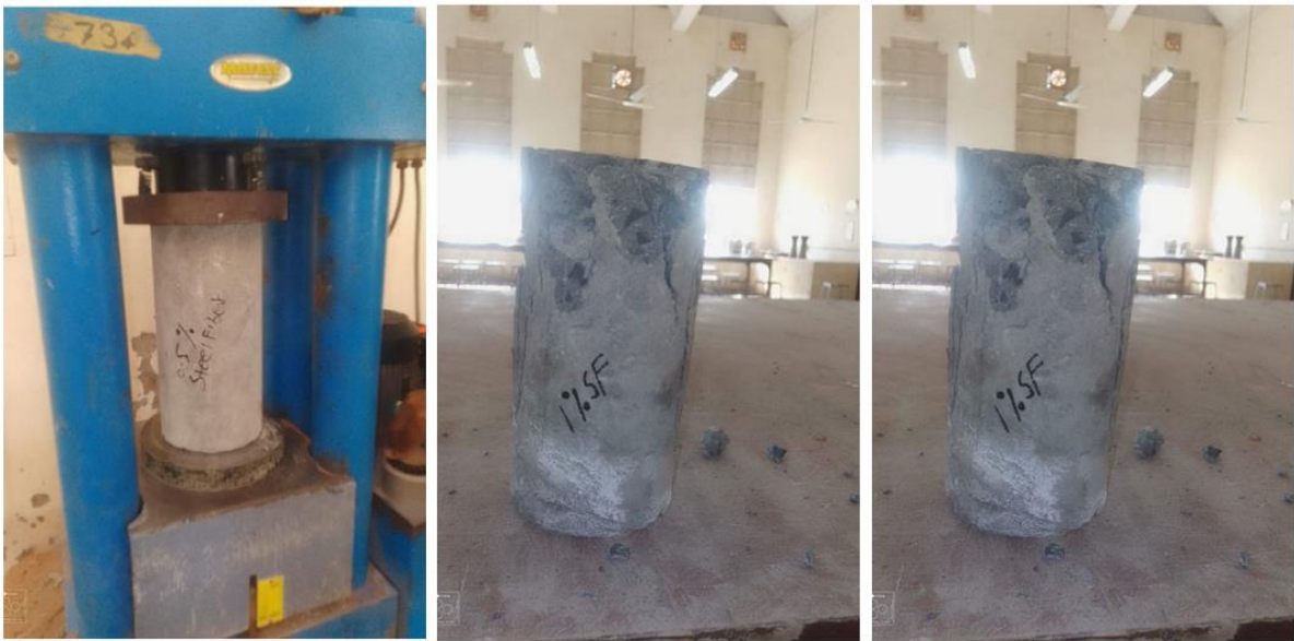
Fig. 4.9 Compressive Strength results of Steel Fiber
