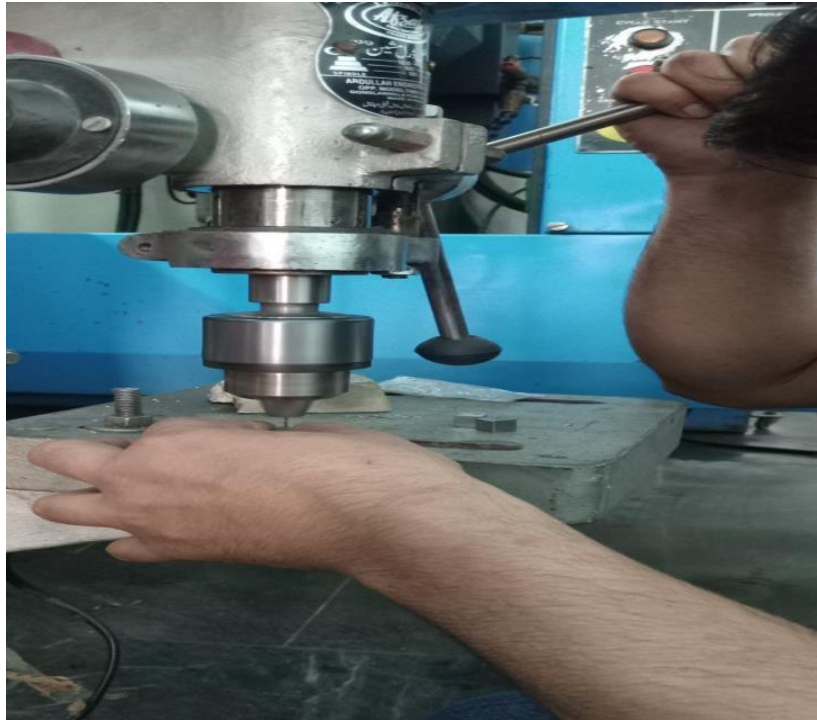
Figure 4 Drilling process on samples for coating
