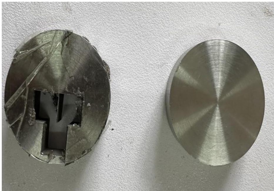
Figure 3 SS316L Samples cut by wire cutting method
