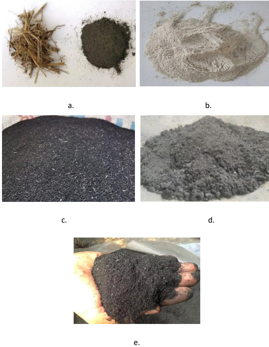
Figure 1 a. Sugarcane/ bagasse ash b. Ceramic powder c. Wheat husk ash d. Corncob ash e. Rice hush ash
