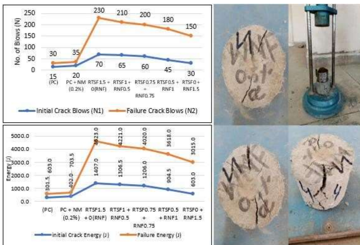
Fig. 6: Overview of Drop Weight Impact Resistance Test & Results
