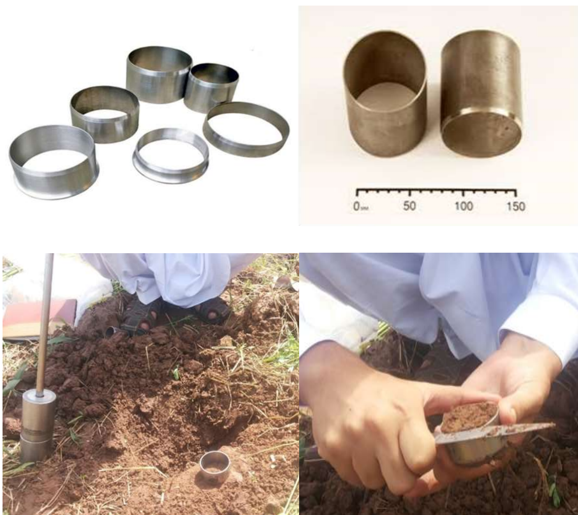
Figure 3. Soil Core Sampling Procedure with different Core Diameters.
