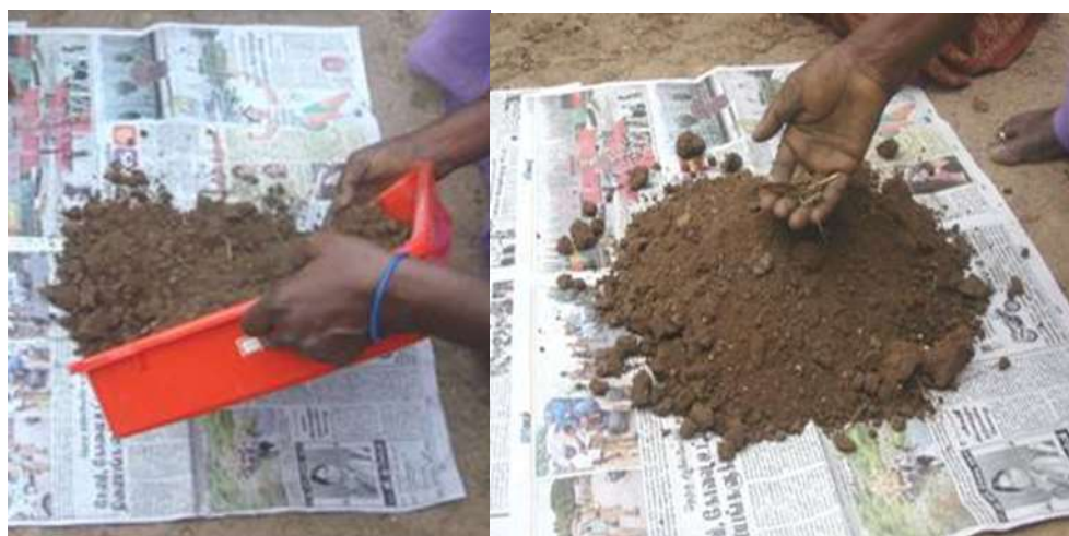
Figure 2. Air Drying And Removal of Materials other than Soil from Soil Sample.
