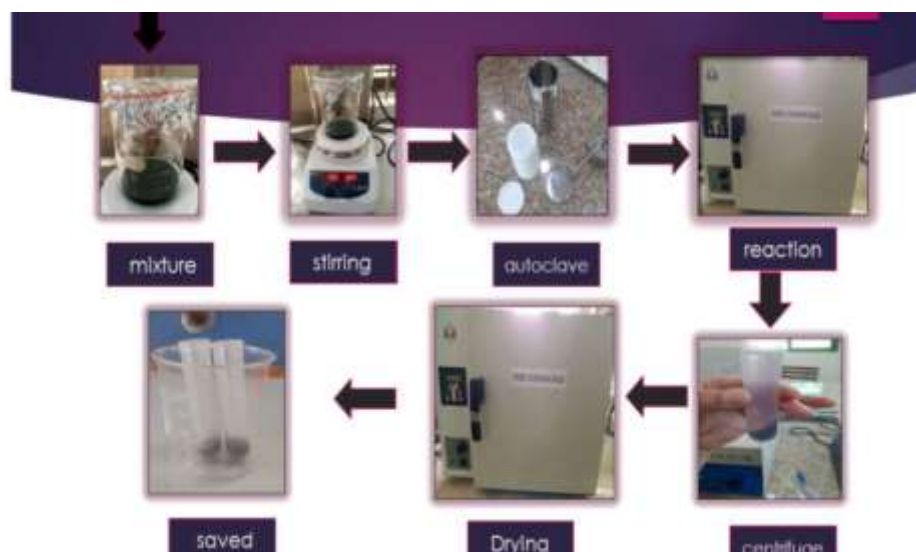
Figure 2.2: Synthesis of Iron Oxide ( \text{Fe}_2\text{O}_3 ) Nano rods
