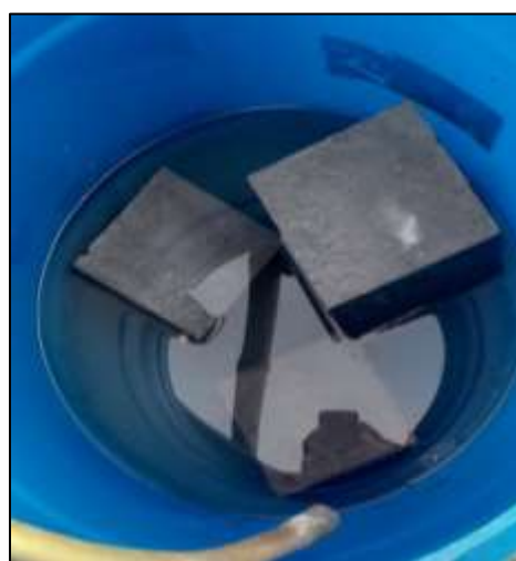
Figure 14. Curing of Concrete Cubes
