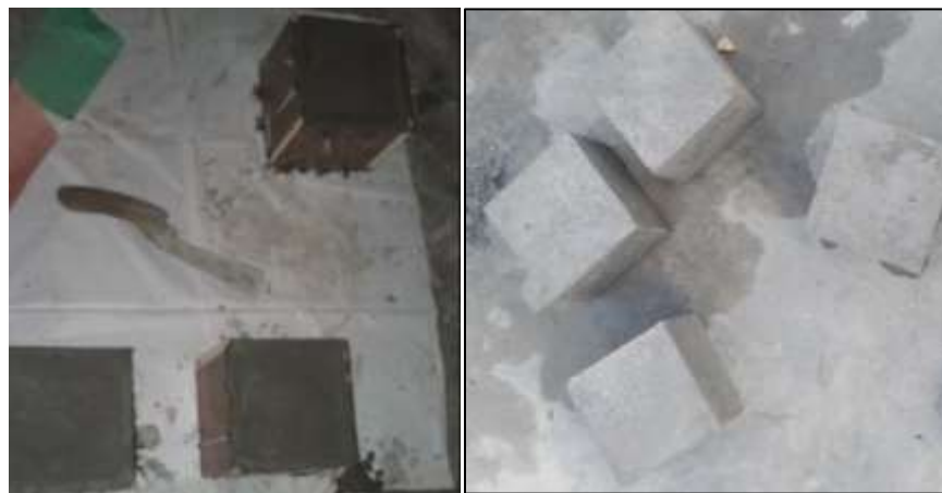
Figure 13. Casting of Concrete Cubes
