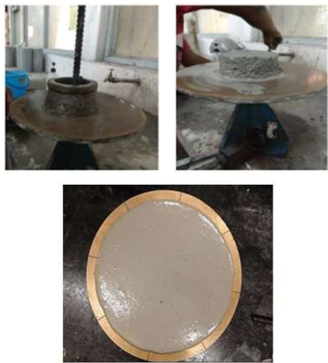
Figure. 2: Workability Assessment of Mortar Using Flow Table Test
