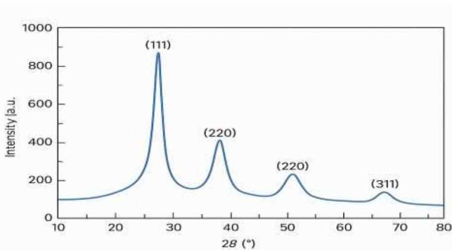
Figure 6. XRD pattern of green-synthesized silver nanoparticles showing crystalline structure.
