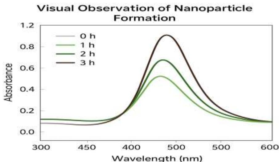
Figure 1. Graph showing the visual change in absorbance spectra corresponding to nanoparticle formation over time.
