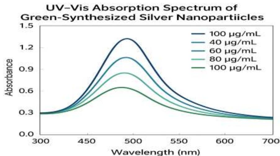
Figure 2. Graph showing UV-Vis absorption spectrum of green-synthesized silver nanoparticles at different concentrations.
