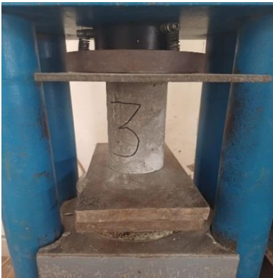
Figure 3 Compressive strength of Concrete
