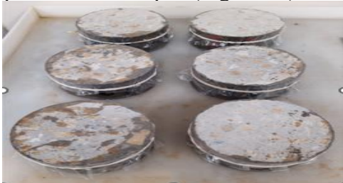
Figure 6 Sorptivity setup for concrete Specimen
