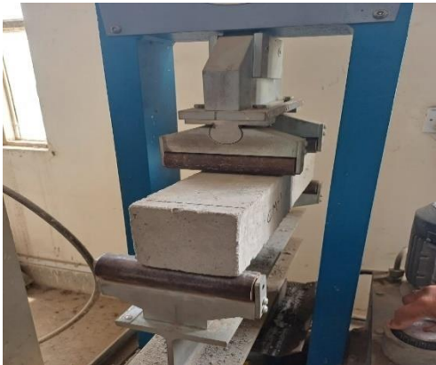
Figure 5 Flexural Strength of Concrete
