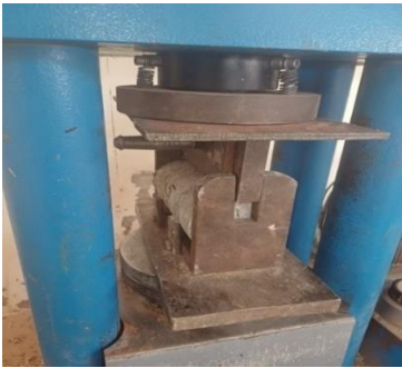
Figure 4 Splitting tensile strength of Concrete
