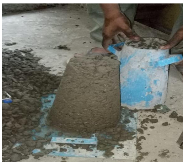
Figure 2 Slump Cone Test
