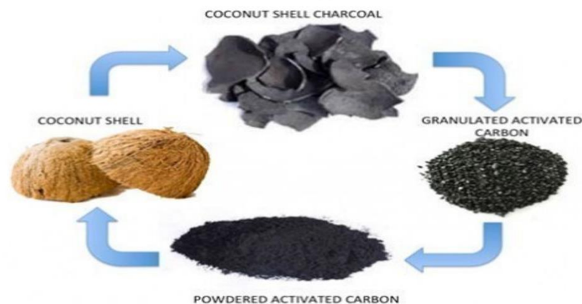
Figure 2: Production of powdered activated carbon from coconut Shell
