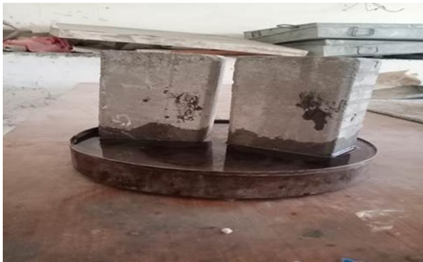
Figure 9: Image illustrating the efflorescence test
