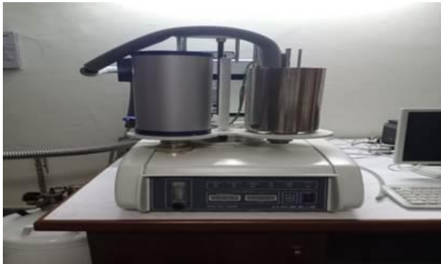
Figure 6: TGA testing machine
