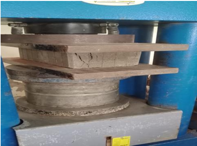
Figure 5: Compressive Strength Test Setup
