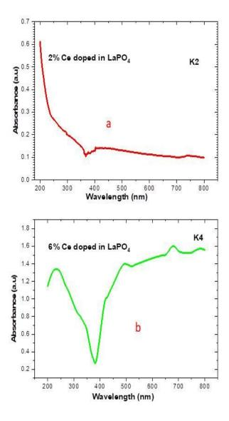
Fig 2.1 (a,b) Band gap of 2% and 6% Ce:LaPO4
