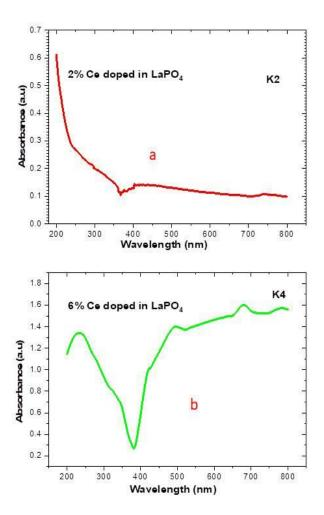
Fig 2.0 (a,b) UV-Visible Absorption Spectra of 2% and 6% Ce:LaPO4
