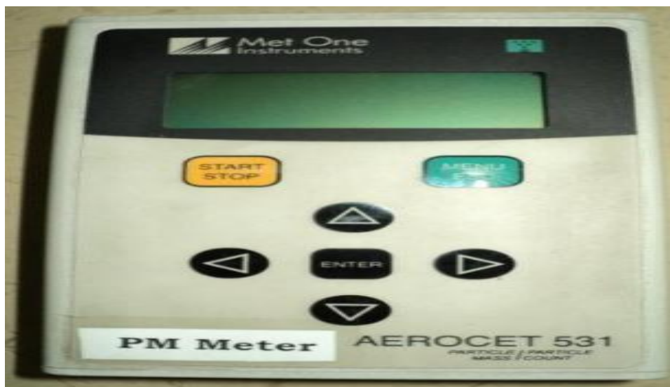
Figure 1 particulate matter emissions measuring device
